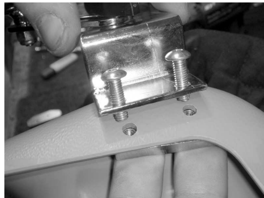
Fig 3 - Line up bracket and mounting block with holes in the shell
